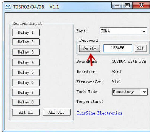
(3) After input the correct password, all the buttons become enabled, then you can control the board now!
