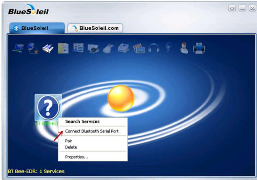
(6) Once your computer have connected with Bluetooth Bee V2, the “STATE” led stops blink. Meanwhile, the device turns green, and BlueSoleil shows “**Connected**”.
