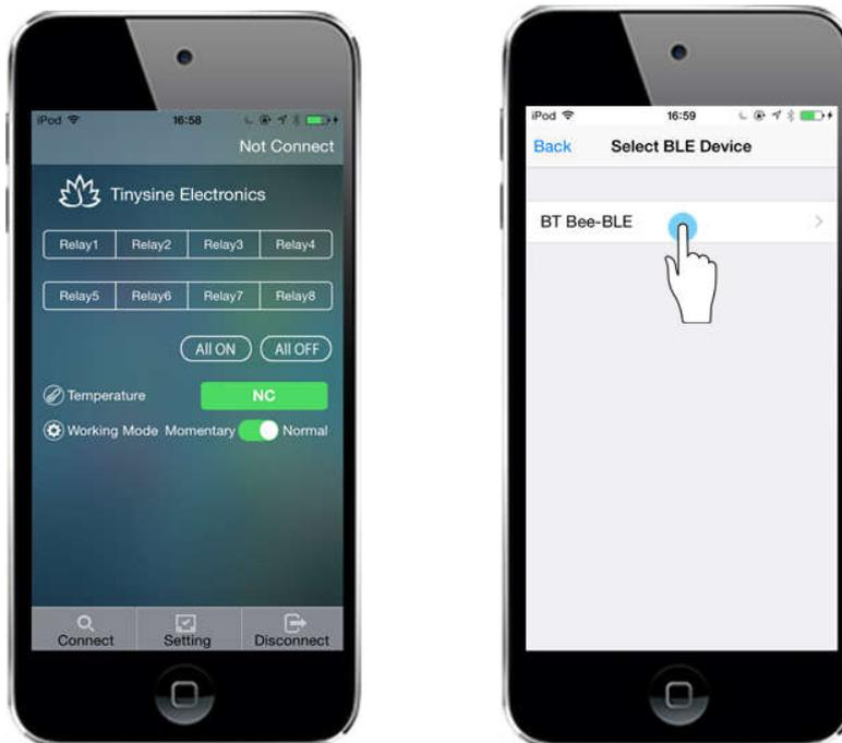
(3) When the app find a device named **“BT Bee-BLE”**, click this device to connect directly
