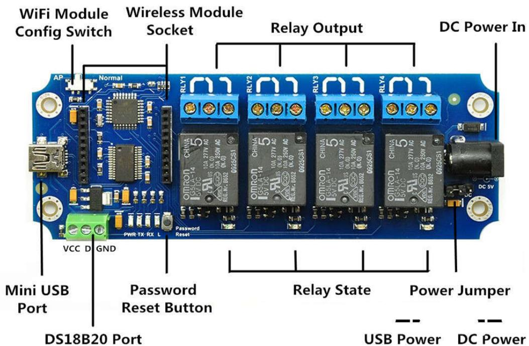
1. Mini USB Port: this port is used to control TOSR14x by computer, or update board's firmware.
