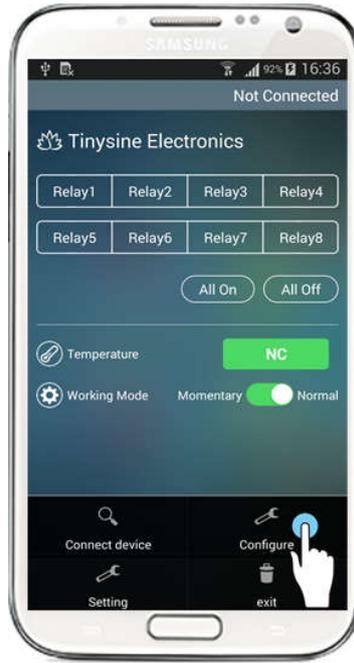
(4) Input your network's settings like SSID, password and IP address in turn, then click "Start". The app will send commands to the WiFi module automatically. Click "Finish" when the app shows configuration is complete.
