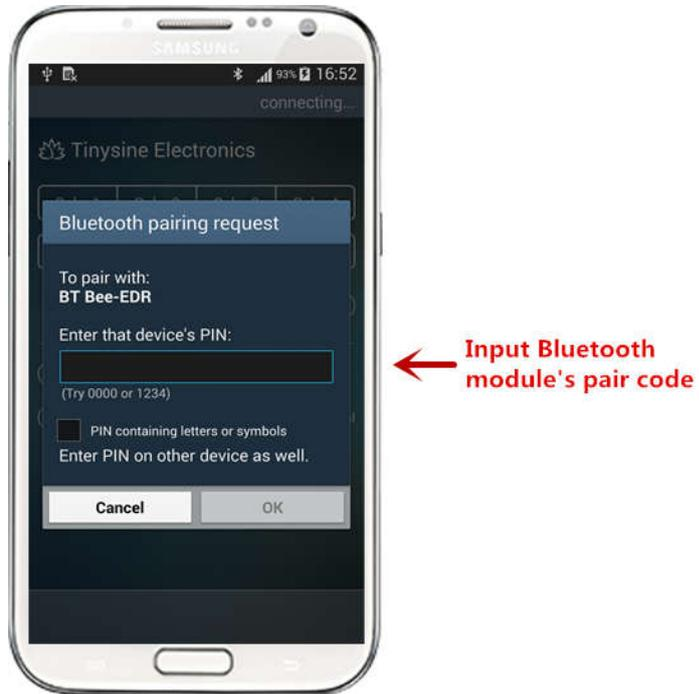
(5) After your phone has connected to TOSR14x, the interface will show **connected: BT Bee-EDR** at the top. Meanwhile, app will ask you for board's password, only when you have input the correct password, you can control the board!
